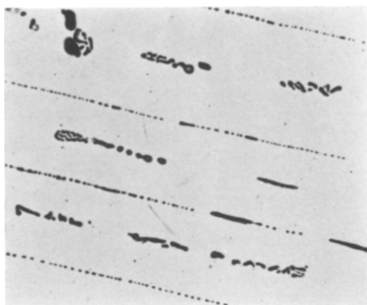
Figure 9 Al-1.5 wt % Sb - R = 22 cm/h. Transverse section. Fine broken lamellae and irregular crystals of AISb ( \times 400 ).
